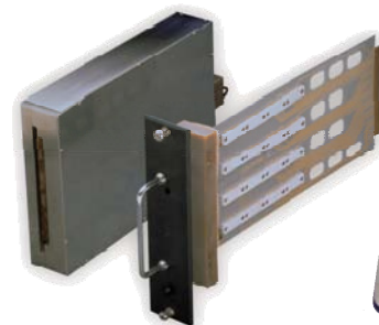
Notebook Oven and High-Temperature DUT Board
