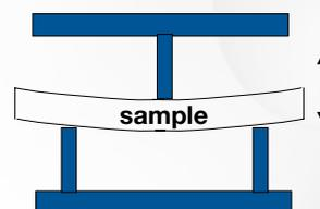
Three Point Bend Test Geometry for DMA
