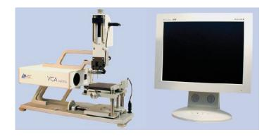
VCA-Optima systems are suitable for research or quality control in R&D and process engineering. Systems range from the basic Optima to the fully equipped Optima XE. Features include dynamic capture capability, motorized syringe, surface energy analysis and pendant drop analysis, to name a few.
