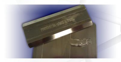
The resultant thin coating or film on the block is then visually inspected for any lumps or non-uniformites on the surface of the coating. Any visual observations can also be read using the scale along either side of the block. This scale can be read in Hegman units (dimensionless), micrometers or mils.
